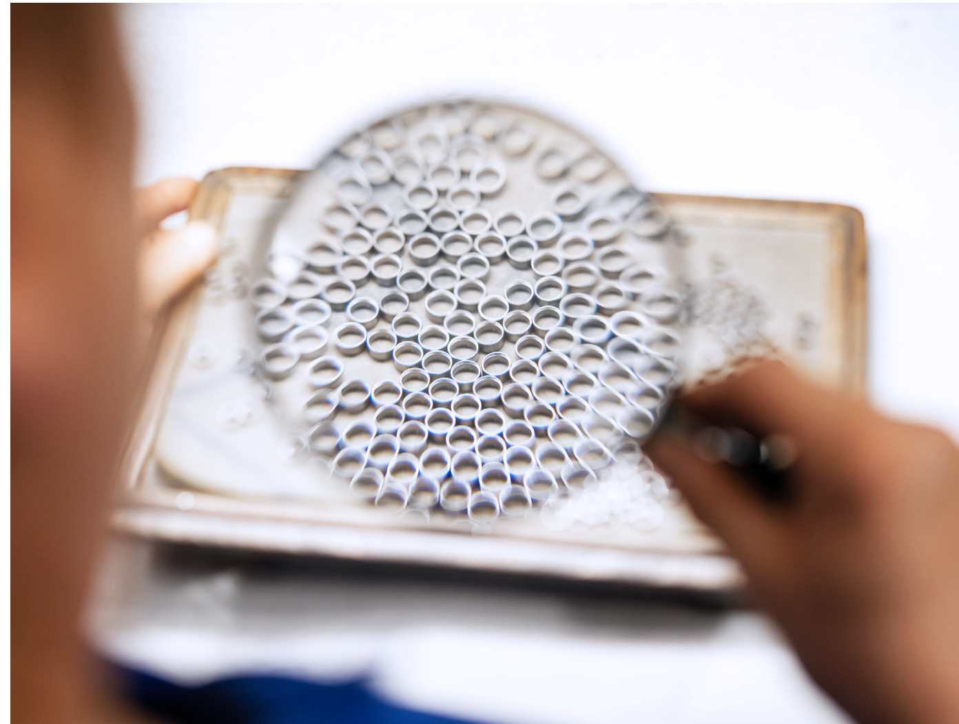
↑ Ball bearing outer rings during visual inspection in production
