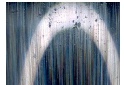
Indentations in raceway caused by particles
